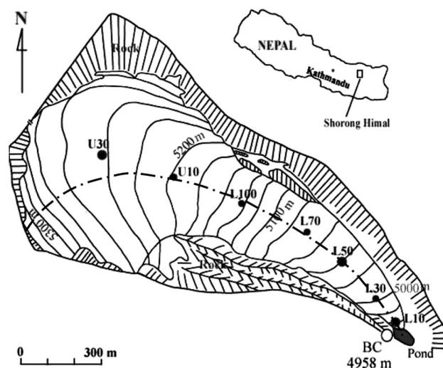
Fig. 1. Location of Shorong Himal and topographic map of Glacier AX010 as surveyed in AD 1978 (Ikegami and Ageta, 1991). Solid circles inside the glacier are positions of mass balance stakes. Solid lines across the glacier are surface elevation contours of 20 m interval. The dotted line along the glacier is the assumed flow line used in the numerical ice-flow model.
