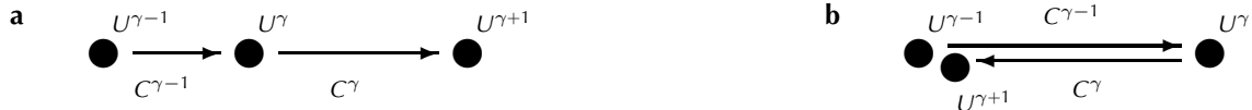
Fig. 1. Illustration of (a) undershooting and (b) overshooting for a sequence of iterates, U^{\gamma-1} , U^\gamma and U^{\gamma+1} , and corresponding correction vectors, C^{\gamma-1} and C^\gamma .
