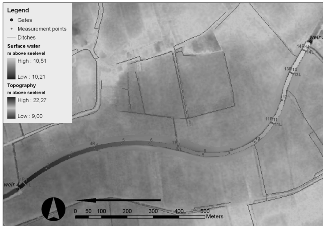
Fig. 1 Digital elevation model showing the examined section of the River Aa close to the town of Herentals, Belgium and the location of the 26 measurement points.
